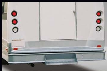
Standard fiberglass rear cap and steel rear bumper with rear step for ease of loading luggage into luggage area
